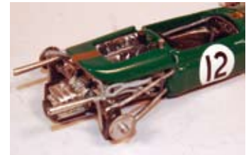
The upper radius rod completes a very busy rear suspension. Note the pipes go above the suspension arms - that's not obvious from the exploded view.
