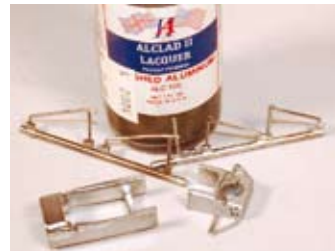
Parts painted with Alclad look good here, but the paint didn't stand up to handling during assembly. A coat of Future floor wax might have solved that.
