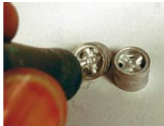
Flash between some of the wheel spokes was easily removed with a sharp knife blade.
