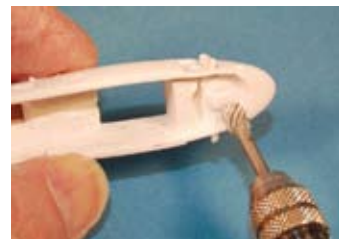
Dremel removes larger pieces of excess resin
